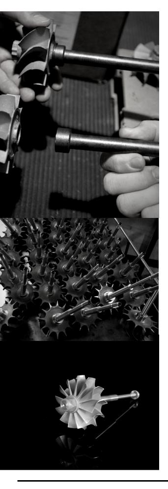
During the process, friction between a rotating and a stationary component causes the two metals to become red hot, at which stage pressure is applied to forge the parts together.
